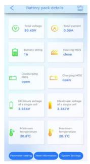
Figure 9: Battery pack details
