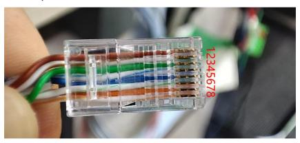
As shown in the figure: no buckle face up, from the top down, the line sequence is 12345678
