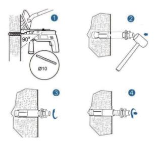
Fig.6-2 Fix the Battery to the Wall
