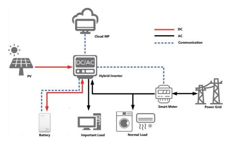
Fig. 3-1 Working Diagram of the Battery Pack
