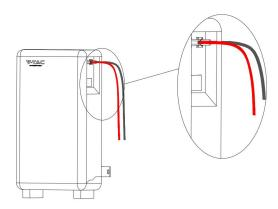
Fig.6-4 Power Cable Connection Diagram
