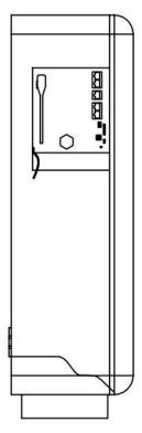
Fig.6-6 GND Cable Connection Diagram
