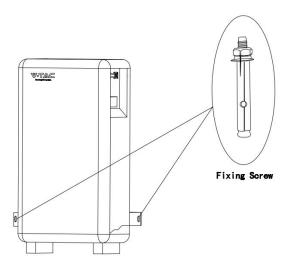
Fig.6-3 Fix the Battery to the Wall
