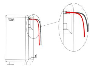
.6-5 Communication Cable Connection Diagram
