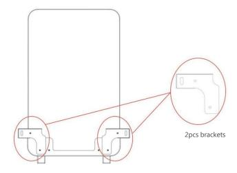
Fig.6-1 Fix the Brackets to the Battery
