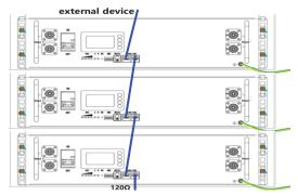
Figure 6-6 Connect 120Ω Resistor
