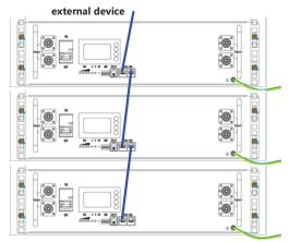
Figure 6-5 Connect RS485/CAN Communication Cable
